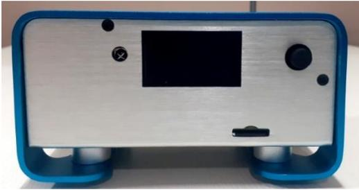
Front : IR sensor, OLED Display Switch, SD card
