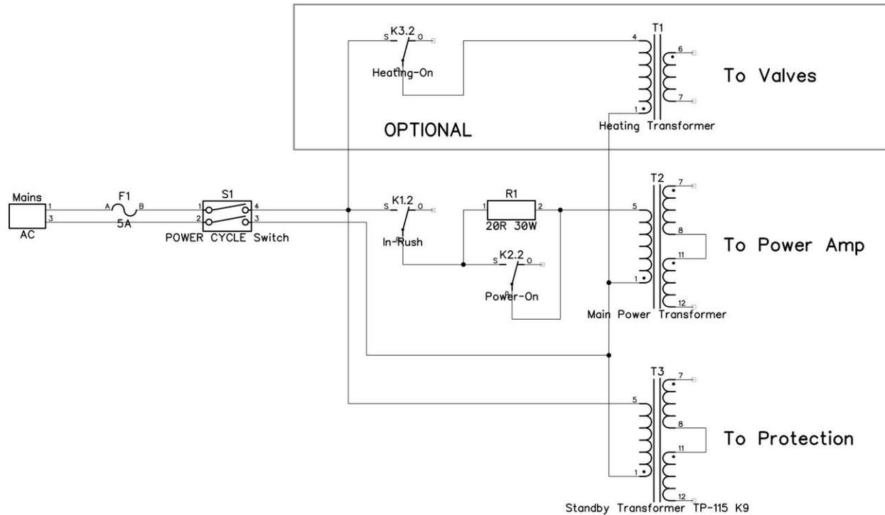
Optional part of the schematic is relevant in case you've got valves in the circuit.
