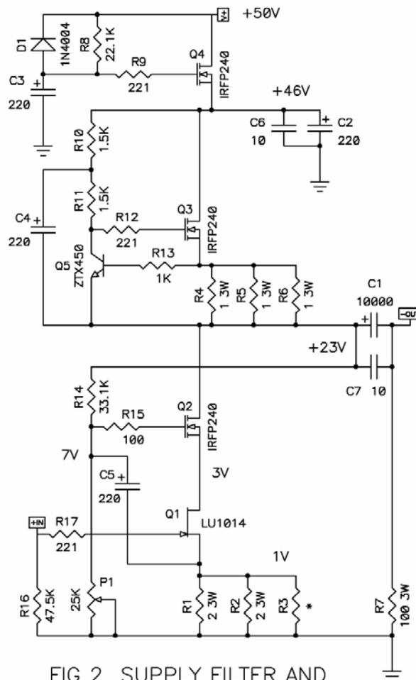
FIG 2 SUPPLY FILTER AND CONSTANT CURRENT SOURCE
