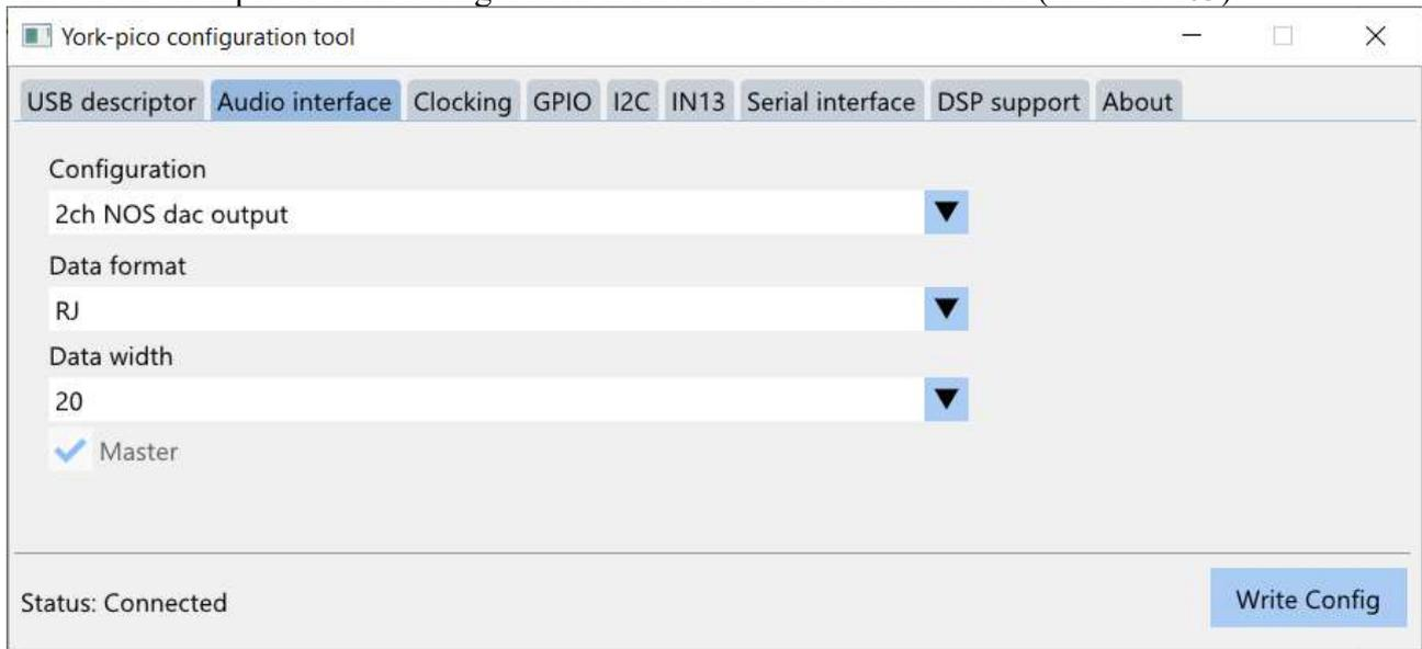
Data width should match with the resolution of DAC IC.
