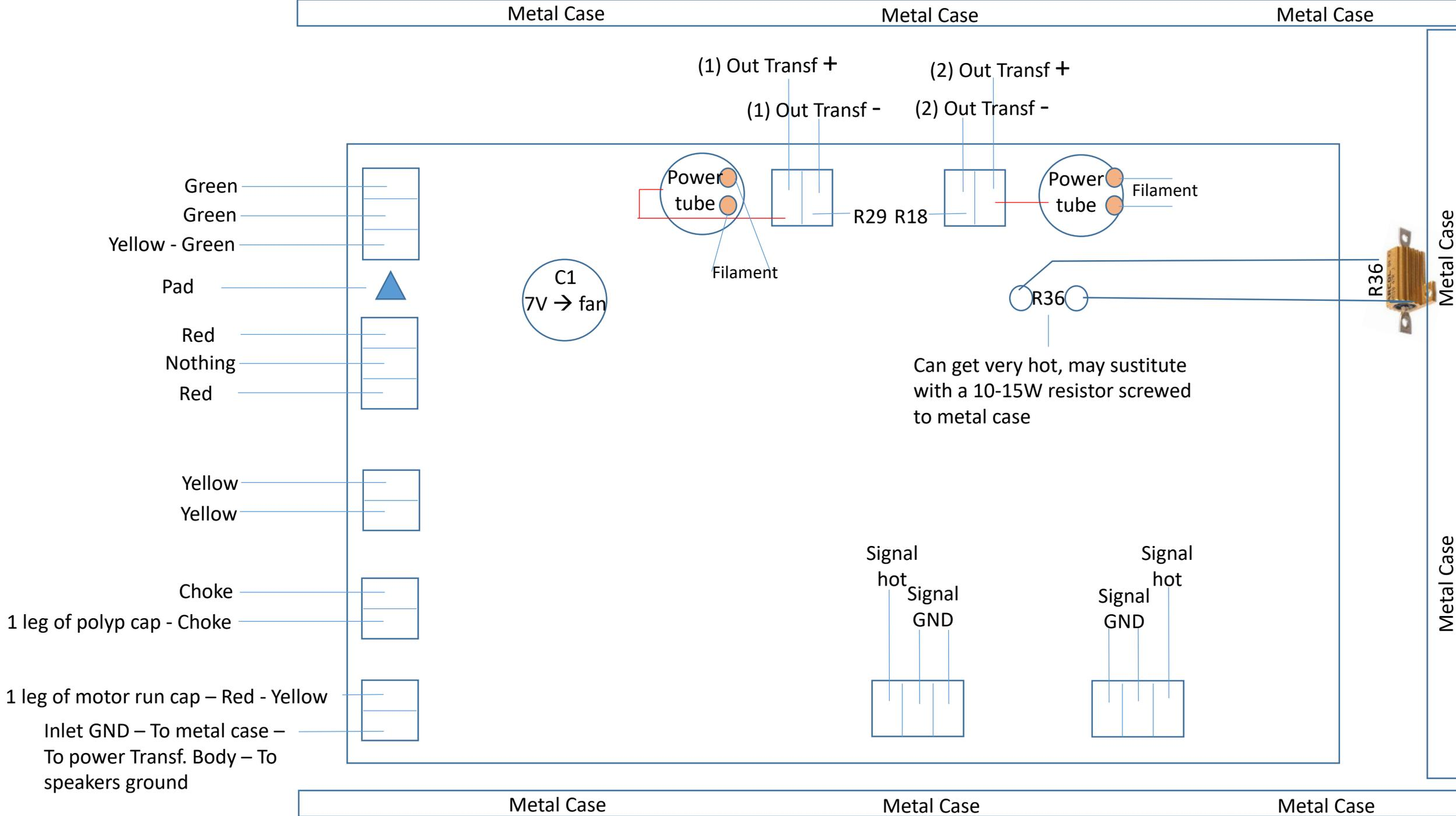
**Without a rectifier** tube installed, the power receptacle was plugged into the Variac and the power was turned up slowly while watching for fireworks/smoke. Filament voltage between pins 2 and 8 measured 5.3 Vac.
