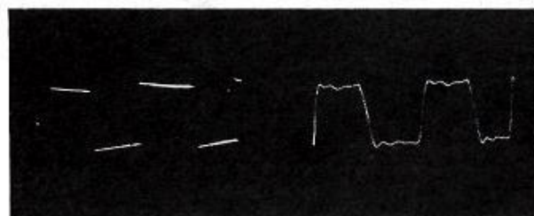
Fig. 3. Square-wave performance at 20 cps (left) and at 50 kc (right).
