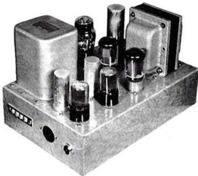
The authors' Ultra-Linear amplifier combined with the power supply on a single chassis.
