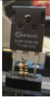
SJEP120R100 inserted in curve tracer socket with 8.3\ \Omega load.
