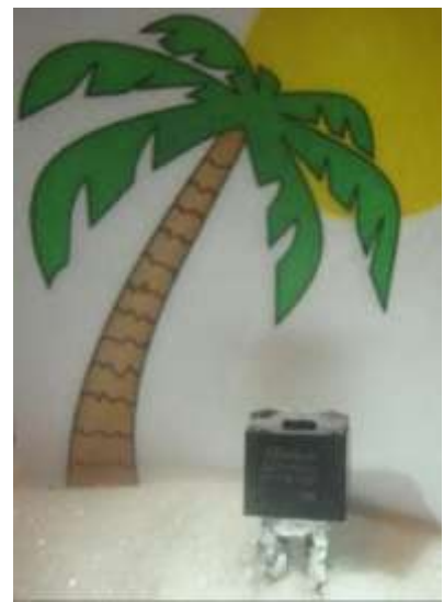
SJD170R1400. This “package” may have short legs, but check out those curves! A normally on, 1.4 \Omega SemiSouth JFET in a TO-263 surface mount package.
