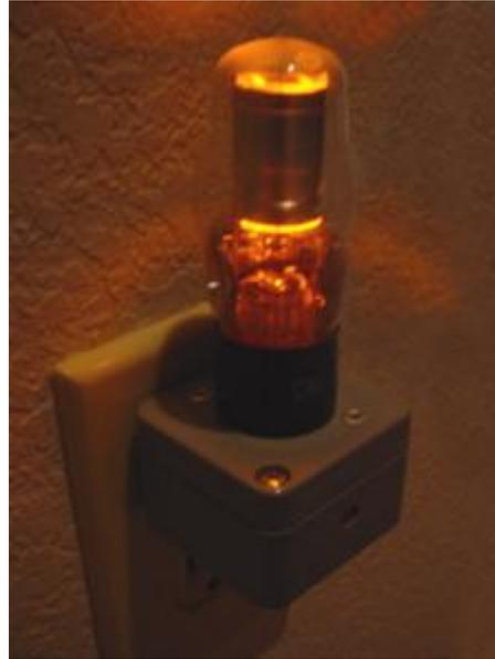
The 0A3 tube is active in both photos, the only difference is the camera's exposure settings. The nightlight will shut off completely in broad daylight.
