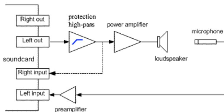
Select Timing: 'Use loopback as cal and timing reference' and 'Merge loopback response into IR' in Measurement window. Check *High pass* in *Preferences Soundcard* if you suspect that DC offset or LF noise damages the measurements.
