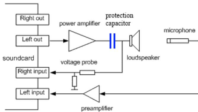
Select Timing: 'Use loopback as cal and timing reference' and 'Merge loopback response into IR' in Measurement window. Check *High pass* in *Preferences Soundcard* if you suspect that DC offset or LF noise damages the measurements.
