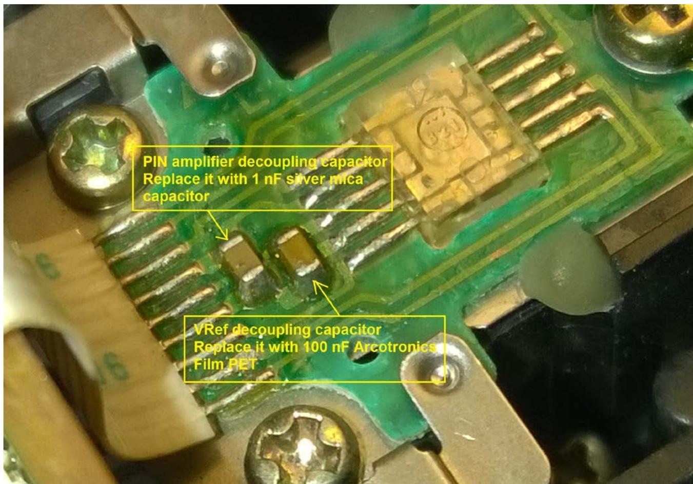
The new capacitors should be [Arcotronics 100nF Film PET](#) and [CD Silver mica 1nF, 100v](#).
