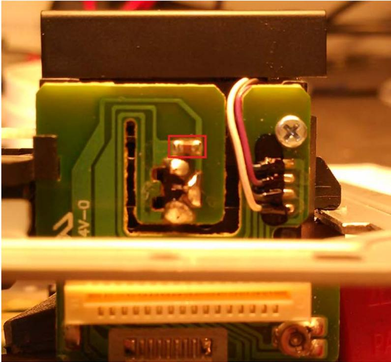
This capacitor must be removed as quickly as possible without overheating the board...
