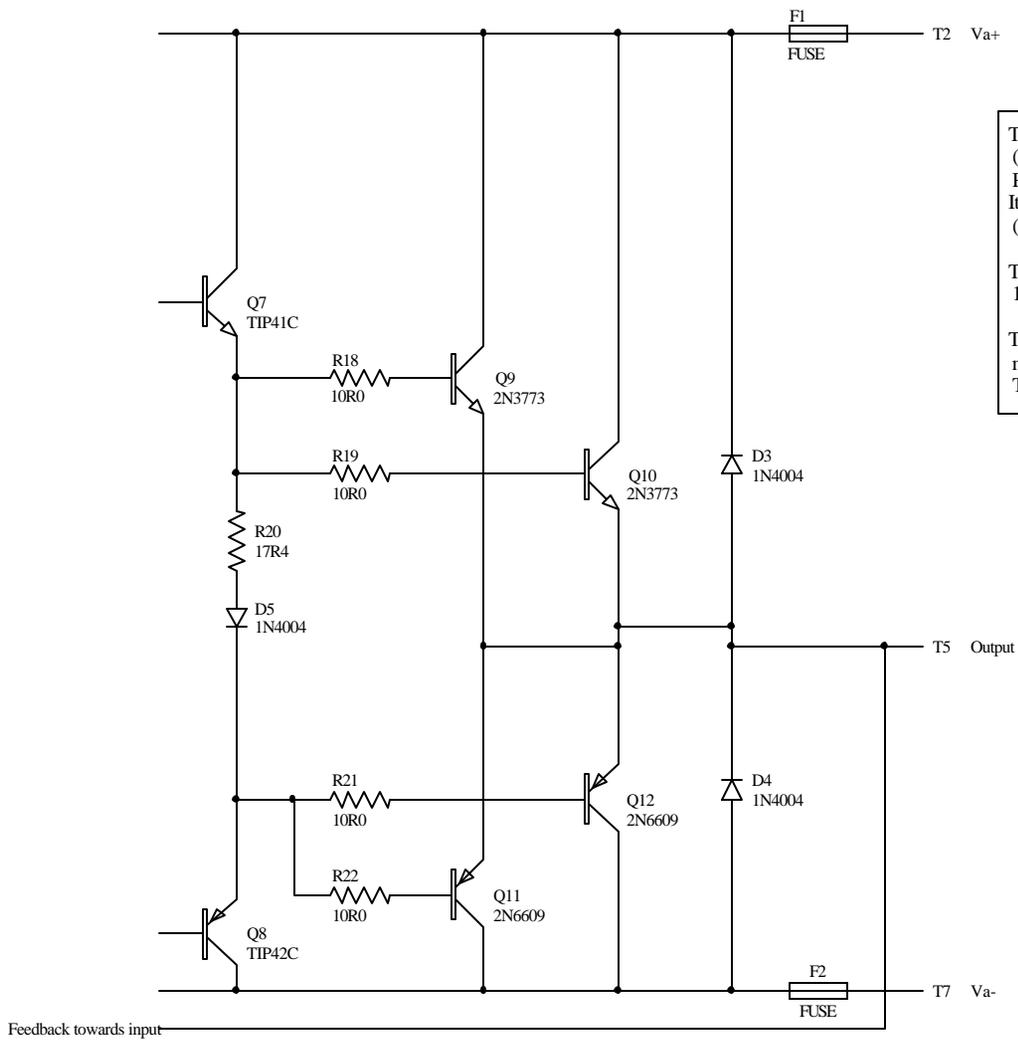
This is the output stage of the VA Systems (aka Van Alstine Audio Systems) Model 3 Power Amplifier. It was nominally rated at 125W in 8 ohms (bridged to 500W).
