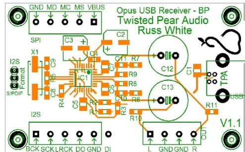
This Opus Receiver Module is based on the Texas Instruments PCM2707. It is mainly intended as a USB audio receiver in conjunction with an Opus DAC module such as the Opus WM8740 module. The module also has a very good built in DAC of its own and can be used completely independently. The device is USB bus powered and requires no other power supply.
