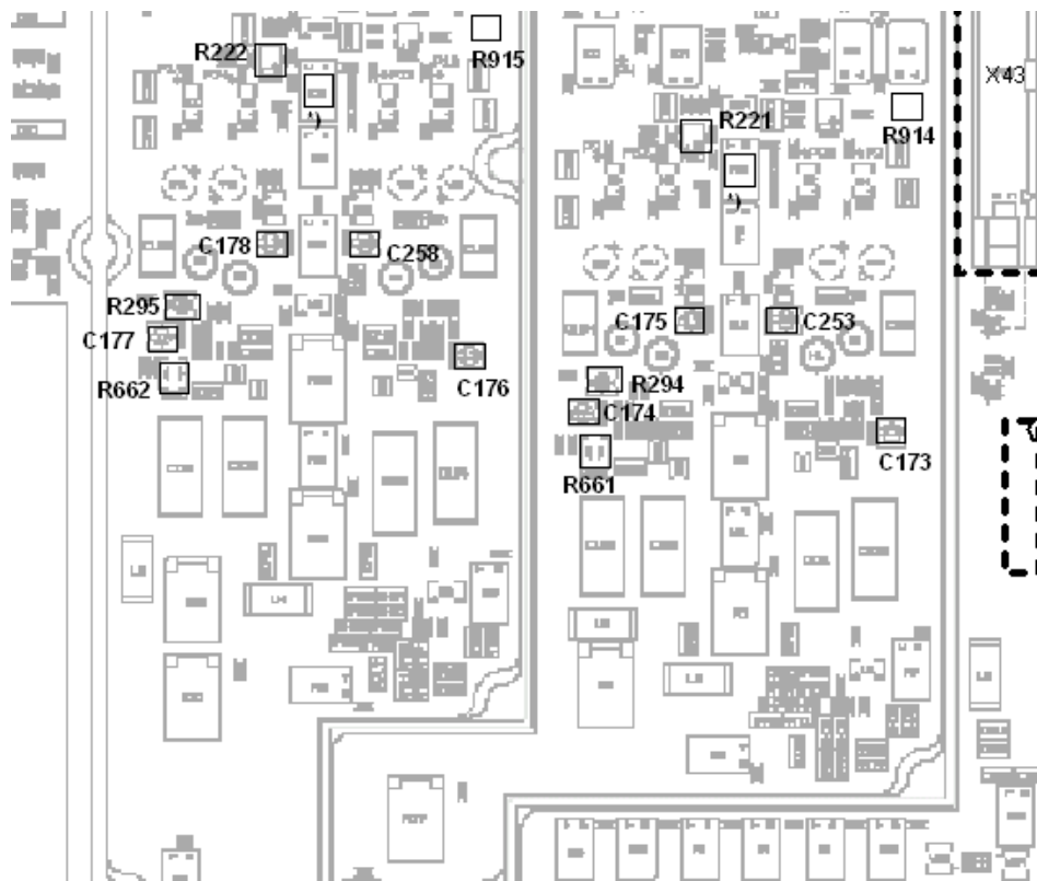
Fig. 2-2 Adjustment Components of Analog Analyzer
