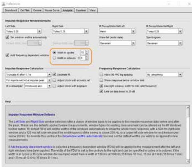
*1/6th octave smoothing and 15 cycles FDW to generate the correction filters and avoid 'micro-managing' the amplitude and phase corrections.*
