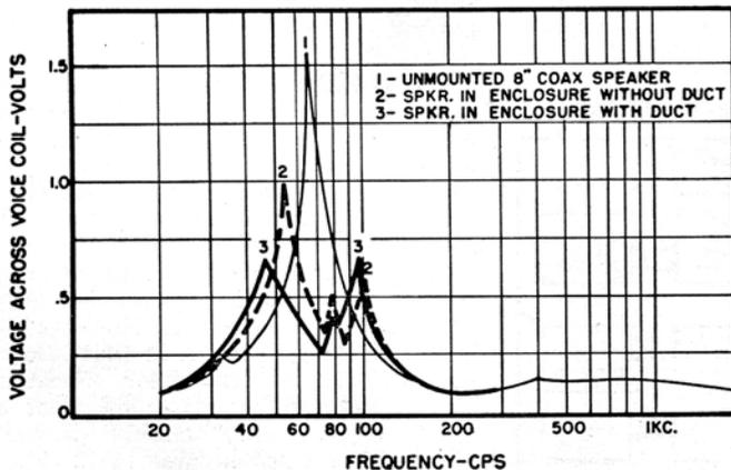
Fig. 2. Impedance curves obtained with 12-inch loudspeaker unit.
