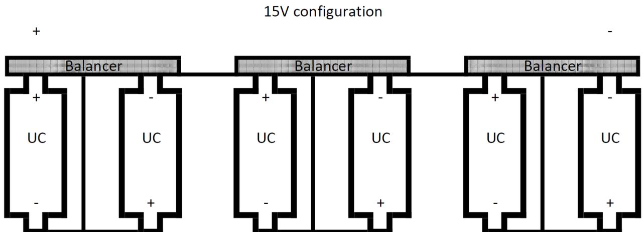
The supplied bridge board needs to be used to configure a ultracapacitor pack with more than two ultracapacitor cells.
