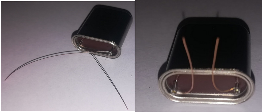
Soldering copper wires to the crystal legs.
