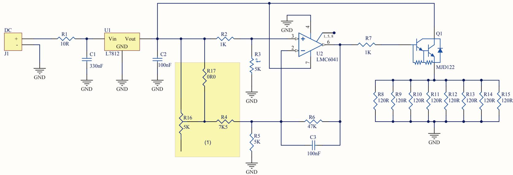
(1) R16 + R4 (7.5 K) for temp fine tuning - R17 + R4 (9.09K) for fixed temp
