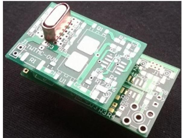
The TWTMC-OVN is the oven to use with SC-Cut crystal oscillators.
