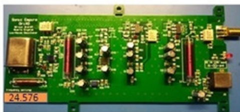
Option 1: fanout both sample rate families
