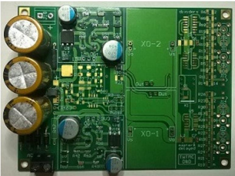
Now you can connect the power transformer to check again the output voltage of the regulators using a DMM.
