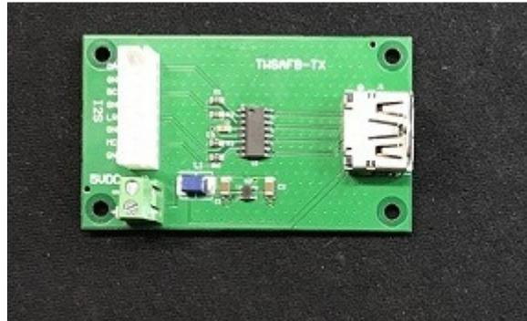
The board transmits I2S signals over HDMI cable. The purpose of this board is to keep the I2S source far from the DAC. The I2S input is single-ended CMOS, the I2S output is LVDS.
