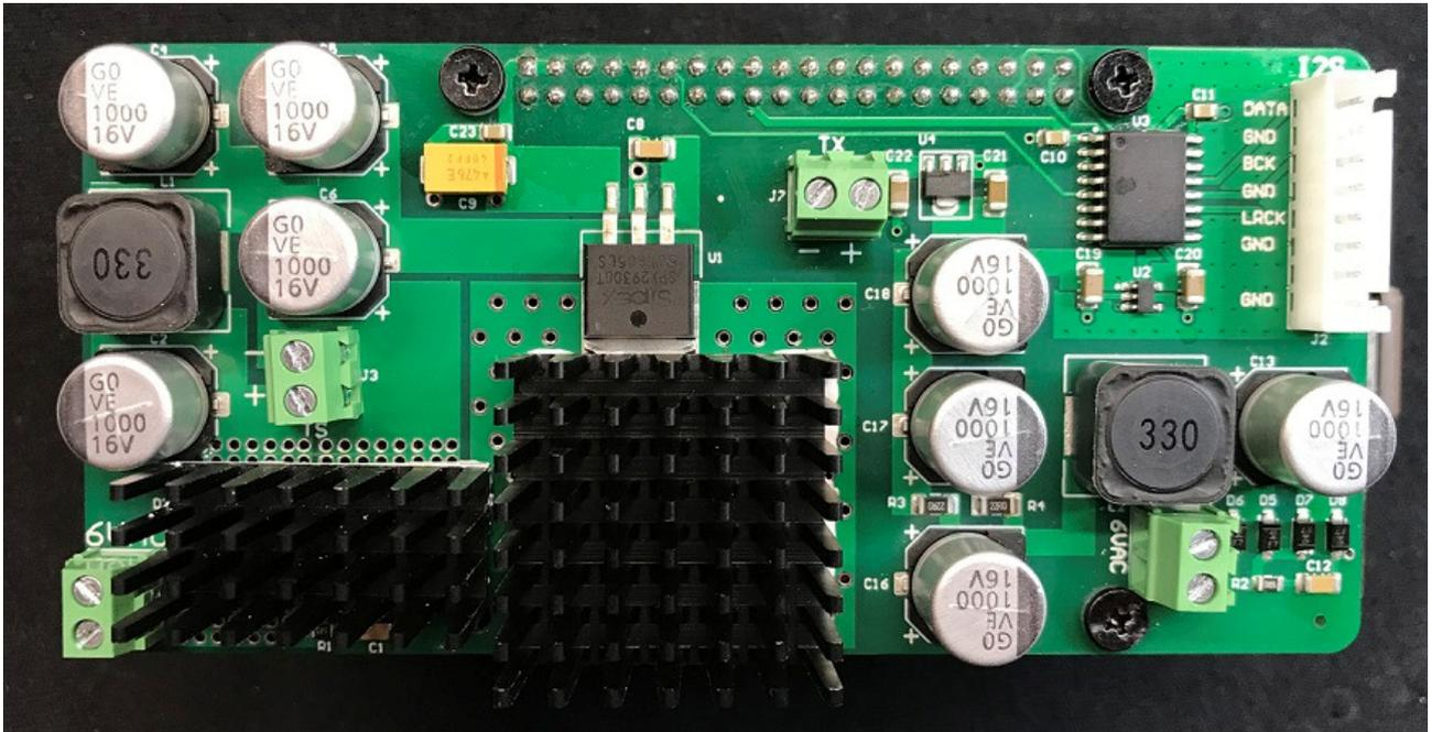
The board is designed to be stacked onto the Raspberry PI. It provides power supply to the RPI and to the official 7" touch screen. It provides galvanic isolated I2S output. The purpose of this board is to build a I2S source from the Raspberry.
