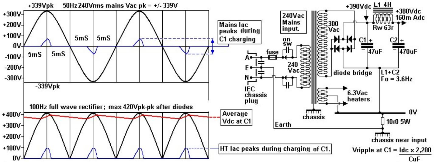
The waveforms in rectifier circuits rectifier should be understood to avoid excessive Vpk across diodes and excessive current peaks. I show a brief schematic for B+ where a 300Vac HT winding makes approximately +380Vdc at 160mAdc at output of CLC filter.
