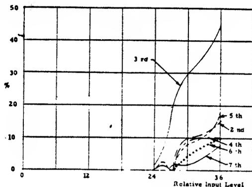
Fig. 10. Distortion components for multistage transformer-coupled transistor amplifier.
