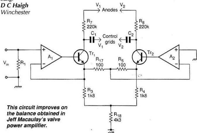
**This circuit improves on the balance obtained in Jeff Macaulay's valve power amplifier.**
