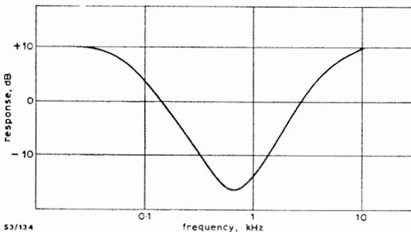
Fig. 4. AMI/11: Response of 40-Hz and 10,240-Hz Circuits Only
