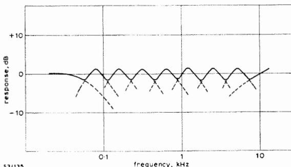
Fig. 5. AMI/11: Resultant Response with All Octave Controls Set at their Mid-points
