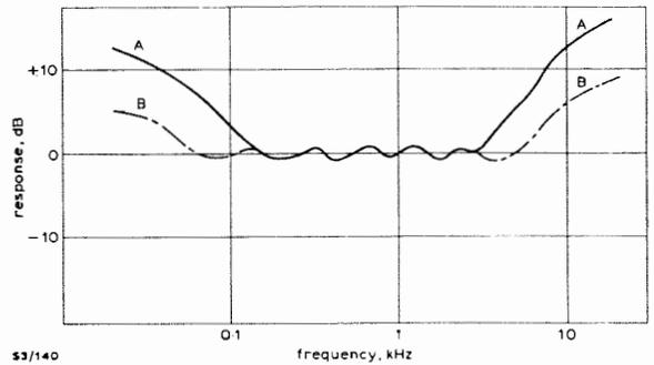
Fig. 10. AM1/11: Response with 40-Hz and 10,240-Hz Controls (A) at  $+14$  dB and (B) at  $+7$  dB. All Other Controls at '0'
