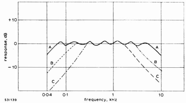
Fig. 9. AM1/11: Response (A) with 40 and 10,240-Hz Controls at  $-14$  dB, (B) with 40, 80, 5,120 and 10,240-Hz Controls at  $-14$  dB, and (C) with 40, 80, 160, 2,560, 5,120 and 10,240-Hz Controls at  $-14$  dB. All Other Controls at '0'
