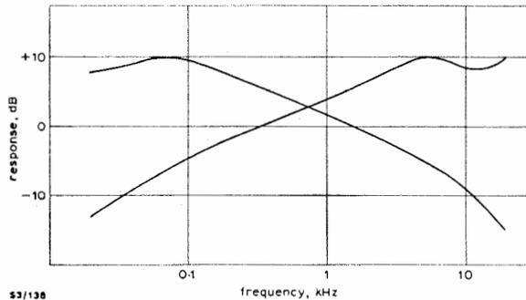
Fig. 8. AM1/11: Response with Control Settings Evenly Graduated Between  $+14$  dB and  $-14$  dB, from 40 Hz to 10,240 Hz and Vice Versa
