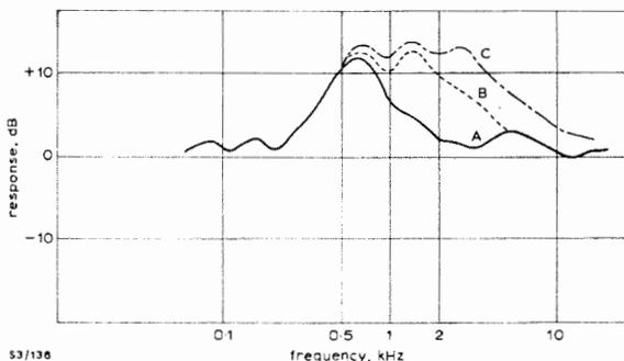
Fig. 6. AMI/11: Response (A) with 640-Hz Control at +14 dB, (B) with 640 and 1,280-Hz Controls at +14 dB, and (C) with 640, 1,280 and 2,560-Hz Controls at +14 dB. All Other Controls at '0'
