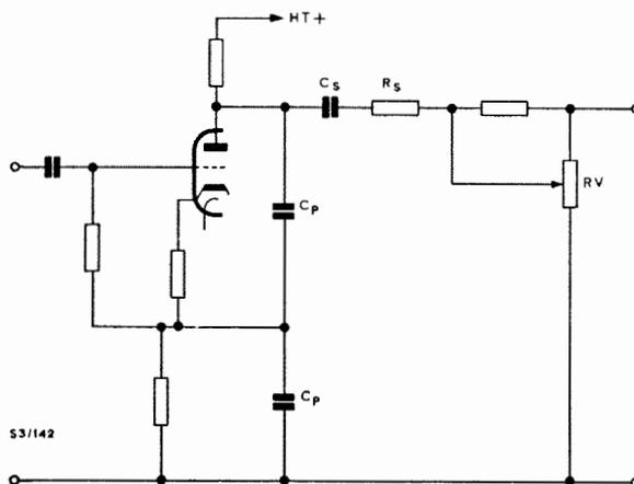
Fig. 2. AM1/11: Circuit of a Frequency-selective Stage
