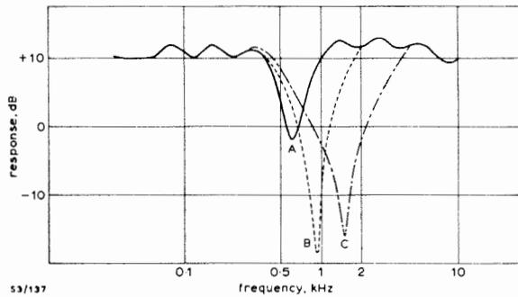
Fig. 7. AM1/11: Response (A) with 640-Hz Control at  $-14$  dB, (B) with 640 and 1,280-Hz Controls at  $-14$  dB, and (C) with 640, 1,280 and 2,560-Hz Controls at  $-14$  dB. All Other Controls at  $+14$  dB. (The shapes of the curves are similar with all other controls at '0' instead of at  $+14$  dB)
