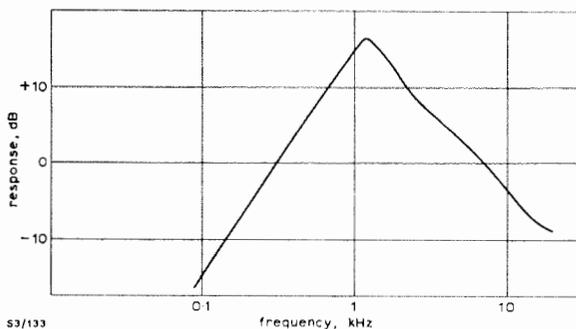
Fig. 3. AMI/11: Response of 1,280-Hz Circuit Only
