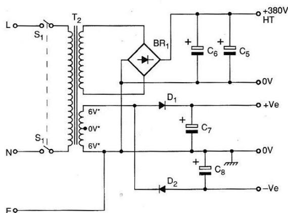
*Being entirely balanced, the amplifier effectively cancels out ripple, simplifying design of the power supply. Voltage for the op-amps is derived from the transformer heater windings. For stereo, two heaters connect to each 6V winding.*
