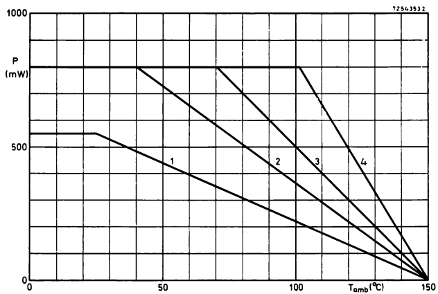
Fig. 4.6. Maximum permissible dissipation over a range of ambient temperatures for various cooling systems:
