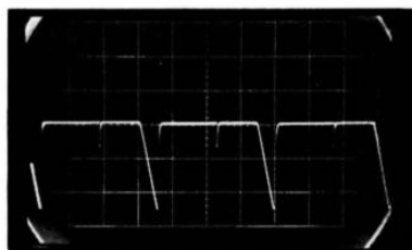
Fig. 3.55. Adjustment of short-circuit Protection Network I.
