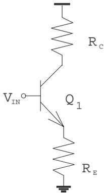
Figure 1: Simplified common-emitter amplifier with emitter degeneration.
