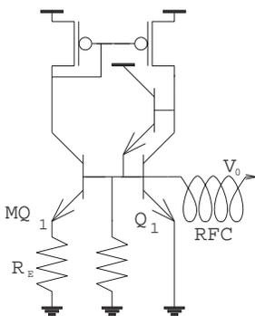
Figure 2: A possible biasing circuit for the common-emitter amplifier
