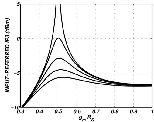
Figure 5: Input-referred IP3 in common-base amplifier for  $R_E = R_S$  and emitter reactance  $L_E \omega_c = 0, 0.05, 0.1, 0.15, 0.2 R_S$ .
