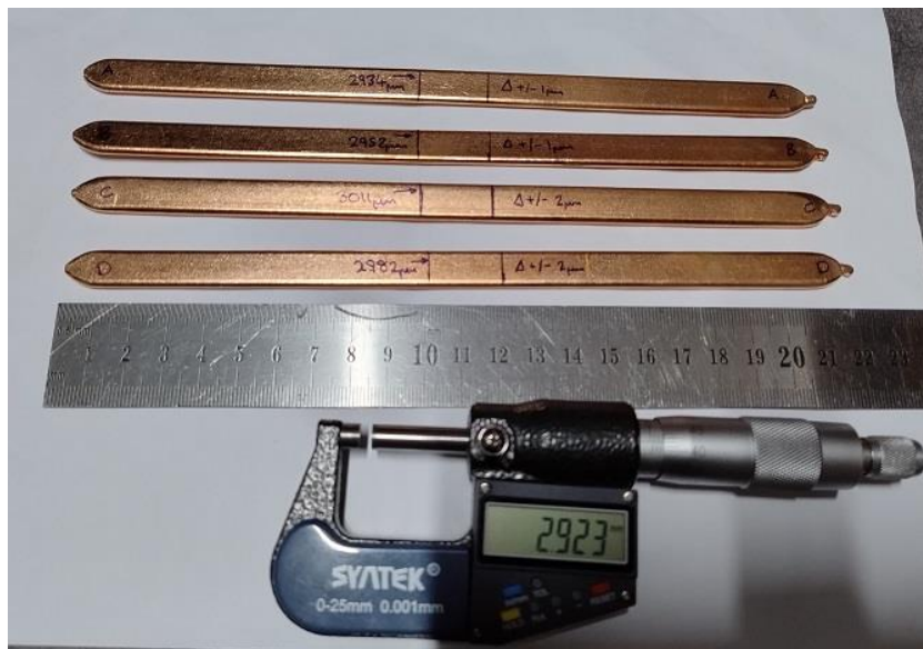
Figure 10. Copper heatpipes used in Experiments 16 and 17.
