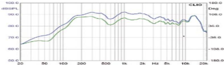
Illustration of a measured array response, un-equalized (blue) and equalized (green)
