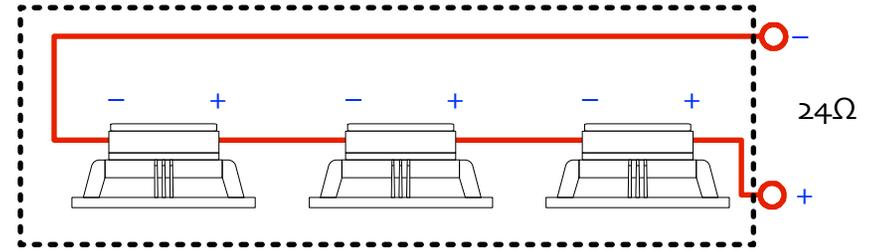
All drivers wired in series, as in a mains module, for an impedance of  $24\Omega$ . Most modern HT receivers will have sufficient power despite a reduction in power to  $1/3$  the rated power into  $8\Omega$ . Note that distortion will also decrease.
