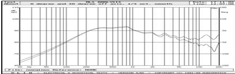
Illustration of a measured array response, un-equalized on axis and 30 degrees off axis
