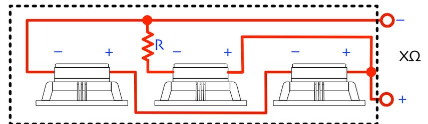
This is a variation of the scheme above (above  $R=0$ ). With  $R=8\Omega$  there is no power tapering and the outer drivers will have the same output as the centre driver (net impedance of the module is  $8\Omega$ ). The resistor will need to be able to handle  $1/4$  the power input. Decreasing the resistor value from  $8\Omega$  will increase the power tapering until maximum is reached when  $R=0$  (as above)
