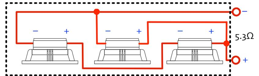
**Recommended:** Outer drivers wired in series, these wired in parallel with the centre driver for an impedance of  $5.3\Omega$ . This will create a tapered array with the centre driver having 3dB greater output than the end drivers.
