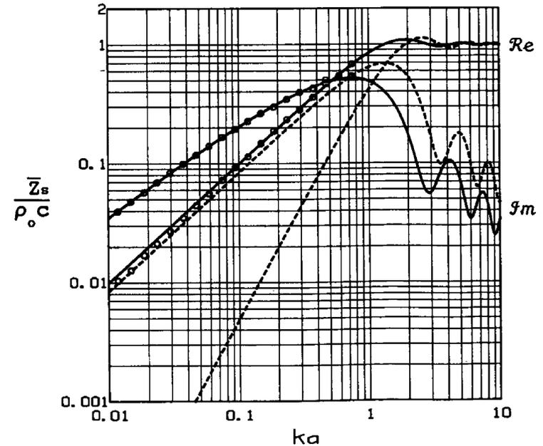
Fig. 4. Comparison of real and imaginary parts of normalized specific acoustic impedance  $Z_s/P_{oc}$  as a function of  $ka$  for one side of: (a) Infinite baffled strip of width  $2a$  (continuous curves). (b) Baffled circular piston of radius  $a$  (dashed curves). Circled points represent numerical computations for finite bar-fled piston of length-to-width ratio 500:1 ( $k = to/c = 2^n/k$ ). [ref 7]
