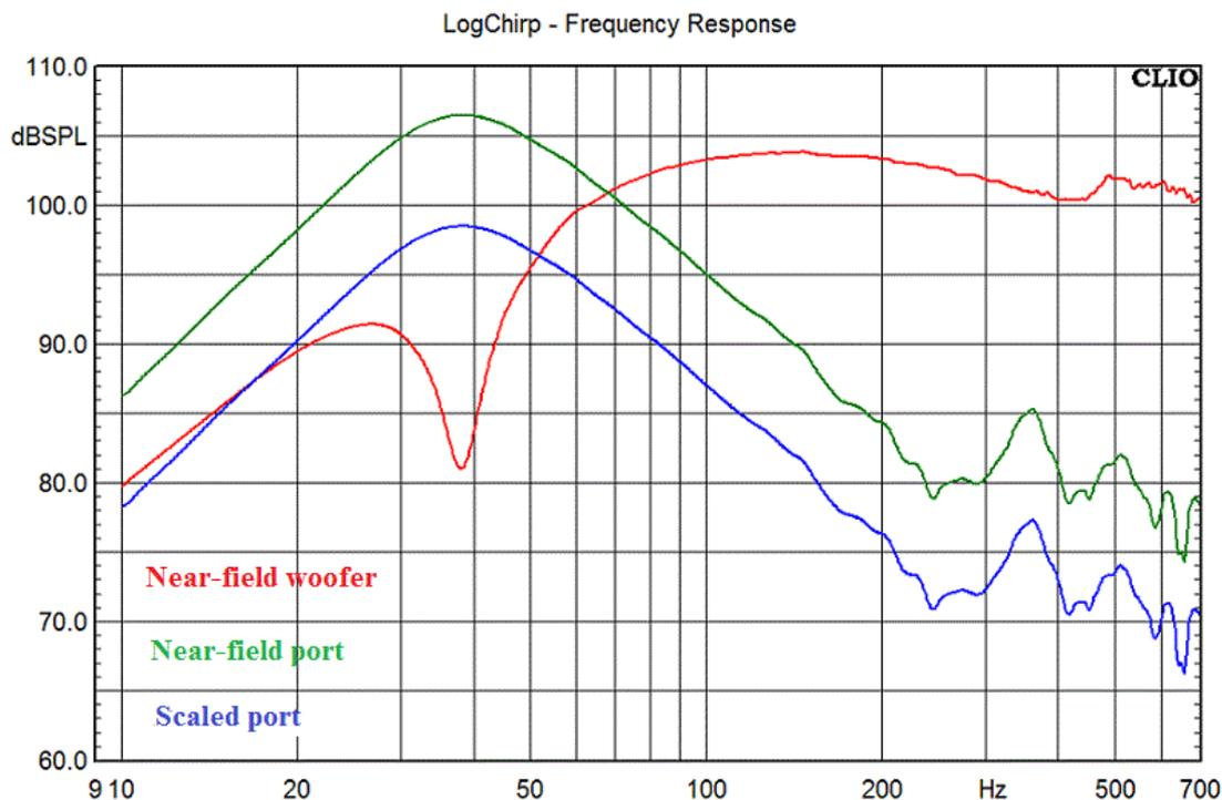
**Fig 4A Near-field woofer, port and scaled port responses**
