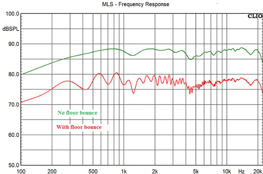
**Fig 3 Two-way frequency response with and without floor bounce**
