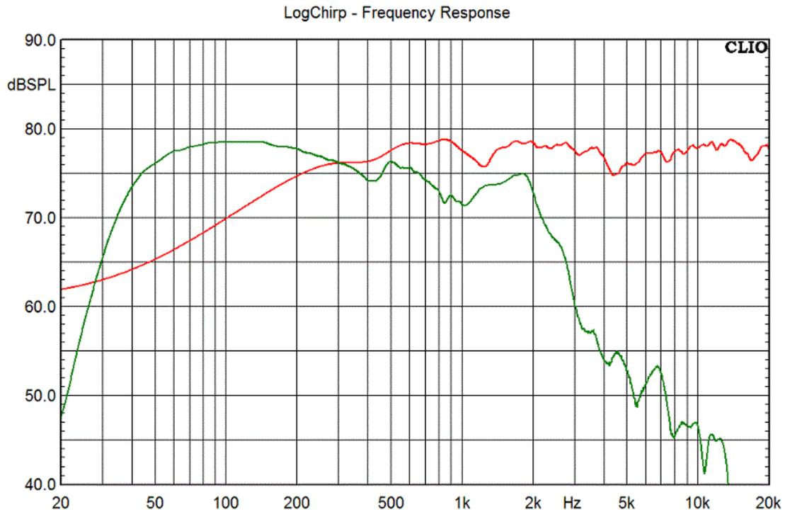
**Fig 5A Two-way fa-field and near-field responses**
