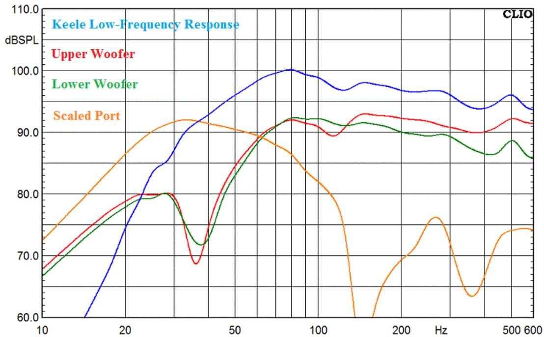
**Fig 16 Tower Speaker Low-Frequency Measurements and Keele Response**
