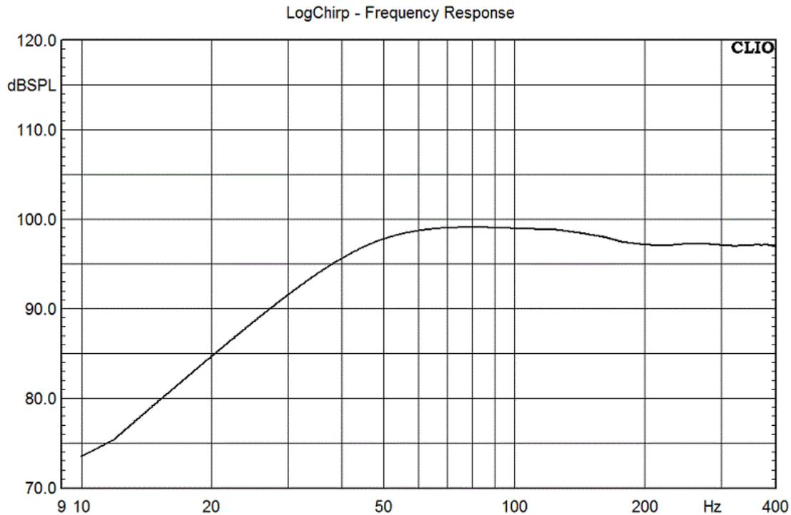
**Fig 11 Subwoofer near-field and MIB responses merged at 150Hz**
