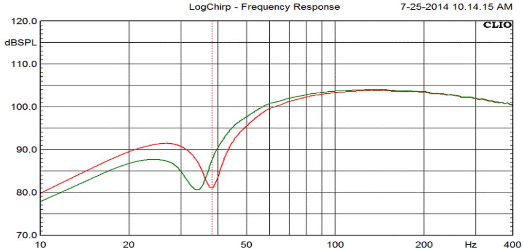
Fig 12 Showing the Effect of Port Contamination on Near-Field Woofer Data
