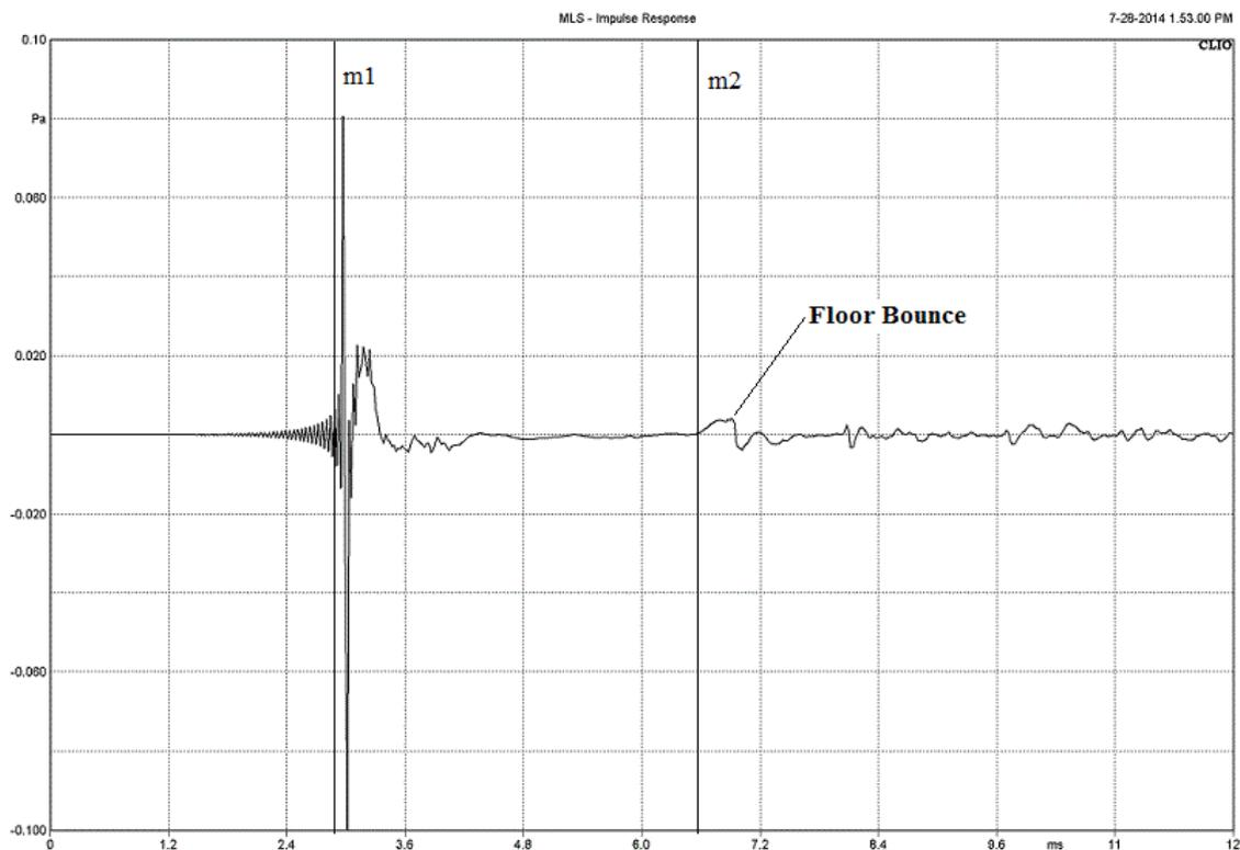
**Fig 2 Measured impulse response of small two-way loudspeaker**
