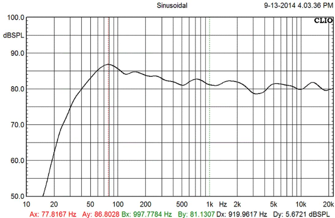
**Fig 17 Tower Speaker Full range response via Keele Approach**
