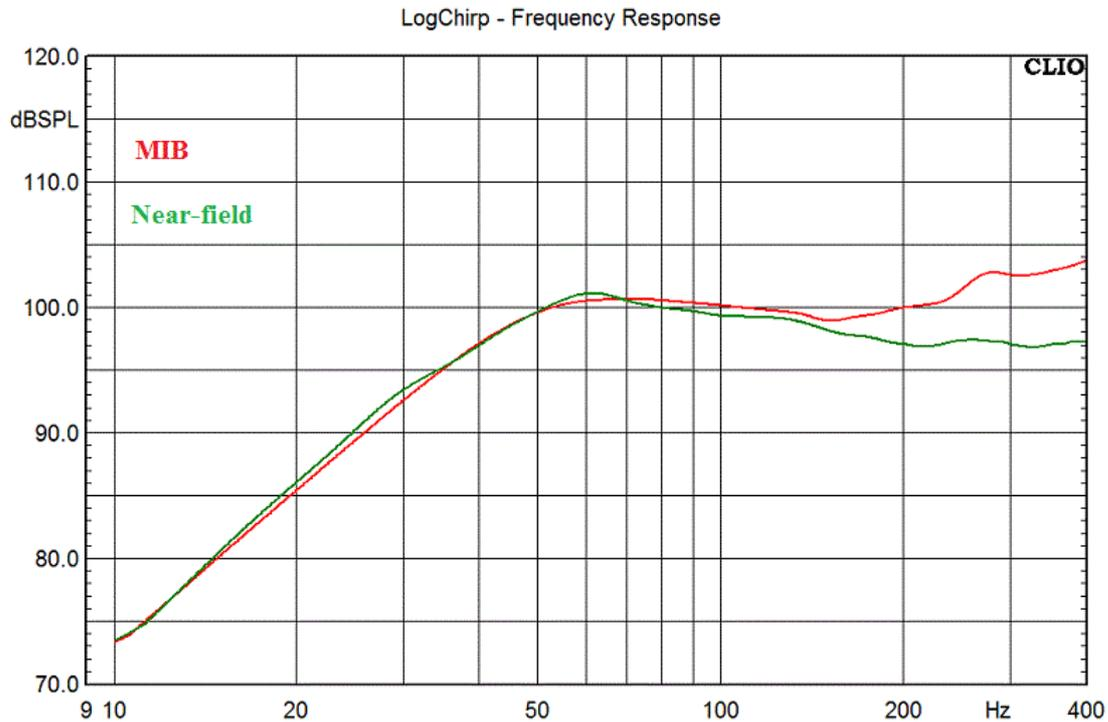
**Fig 10 Comparing MIB and near-field subwoofer responses**
