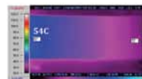
TC1050 Composite 45W heater 20° chill block
