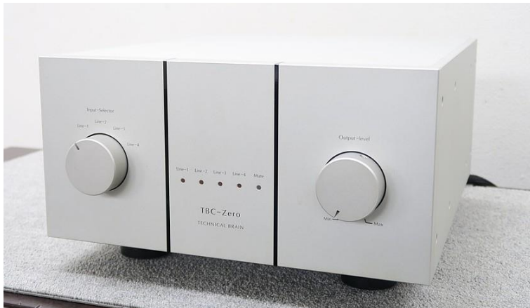
[Photo 2] Front appearance of the preamplifier TBC-Zero released in 2005 (the price at the time of release is 1.7 million yen excluding tax). The knob has a volume on the right and an input selector on the left. In the centre are four input sources and muting indicators lined up in a row
