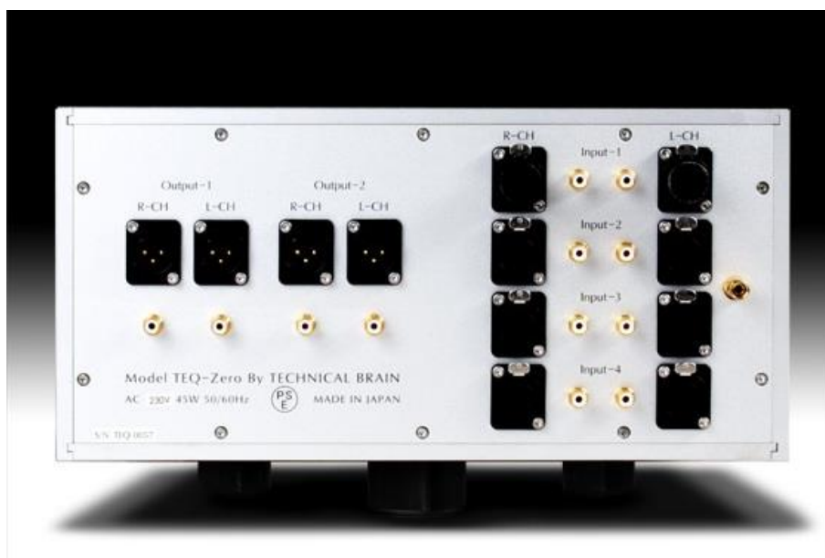
[Photo 12] TEQ-Zero's rear panel. Same as TBC-Zero except that the ground terminal is added. The right column is the 4 input terminals of the system. The left is the output of the system. The XLR terminals can be connected in parallel with the adjacent RCA terminals.
