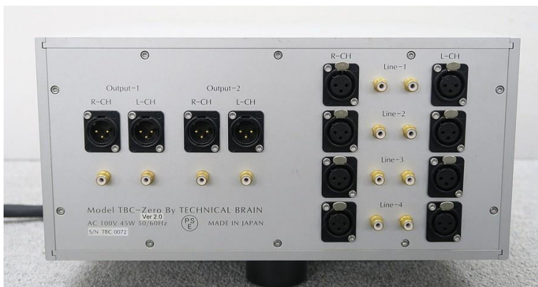
[Photo 3] Rear panel of TBC-Zero. The right column are the 4 input terminals, the left are the 2 outputs. The XLR terminal is hot at Pin 2 and is connected in parallel with the adjacent RCA terminal.
