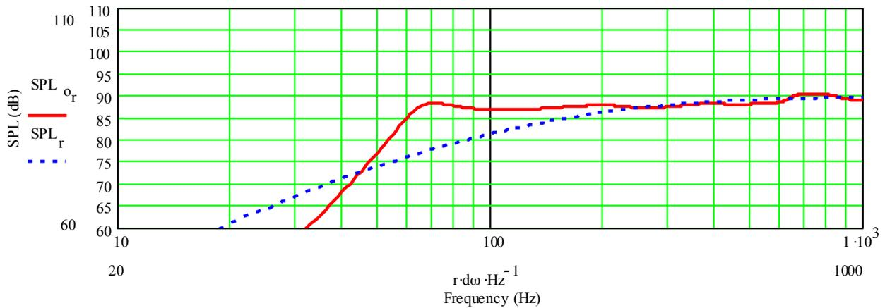
By reducing the port length, the tuning of the enclosure will raise. This adjustment will give you a better result. There is more output from 200 Hz and below.
