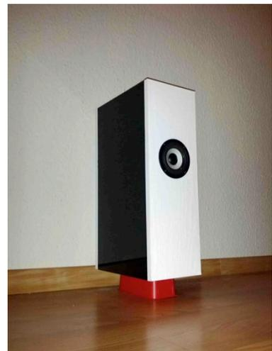
The sides are 9 mm plywood and 3 mm black Acryl in my cabinet. You can place the cabinet upside down or any other position as long as the opening is not blocked.
