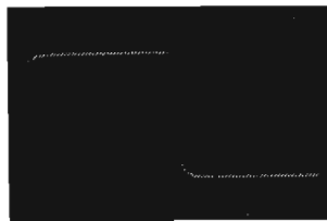
Fig. 10B. Transient response, high level, tuner-to-line. [Tone controls off]. 10kHz, 5V/cm V; 10uS/cm H.
