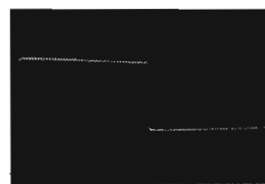
Fig. 7C. Transient response, phono-to-tape. Through precision inverse RIAA equalizer; 60kHz bandlimit. 1kHz, 0.5V/cm V; 100 \mu S/cm H.
