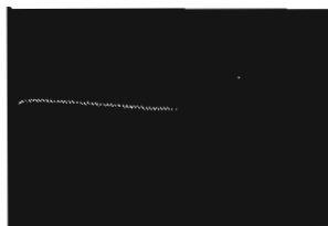
Fig. 7D. Transient response, phono-to-tape. Through precision inverse RIAA equalizer; 60kHz bandlimit. 1kHz, 0.2V/cm V; 100 \mu S/cm H.
