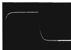
Fig. 7E. Transient response, phono-to-tape. Through precision inverse RIAA equalizer; 60kHz bandlimit. 10kHz, 0.5V/cm V; 10 \mu S/cm H.
