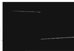
Fig. 10A. Transient response, high level, tuner-to-line. [Tone controls off], 20Hz, 0.5V/ cm V; 5mS/ cm H.
