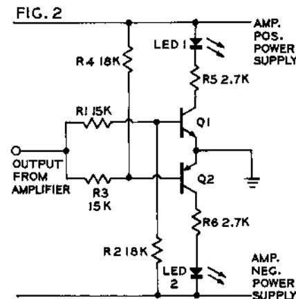
power-supply provides a convenient means of establishing a specific reference for any size amplifier, large or small, as well as sensing the instantaneous value of the supply-voltage, which tends to rise and fall somewhat depending on load and power-level.
