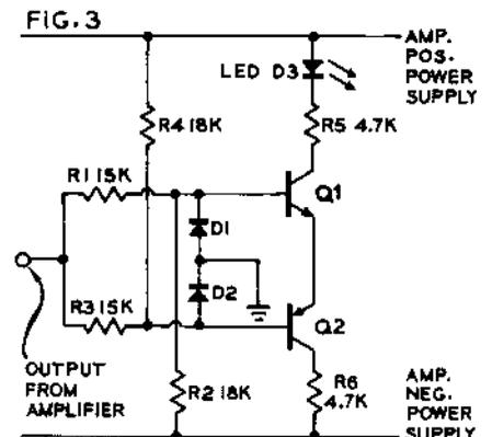
almost universal, and it may be used with nearly any solid-state power amplifier or amplifier section of a receiver. In some low-powered amplifiers (below 50 W/chan.), the circuit may not operate due to insufficient voltage for triggering. This can be solved by substituting a slightly lower value, say 15K, for resistors R1 + R3, and changing R5 + R6 to 2.2K. 10K 1W resistors are advised for R5 + R6 with amplifiers over 300 W/chan.
