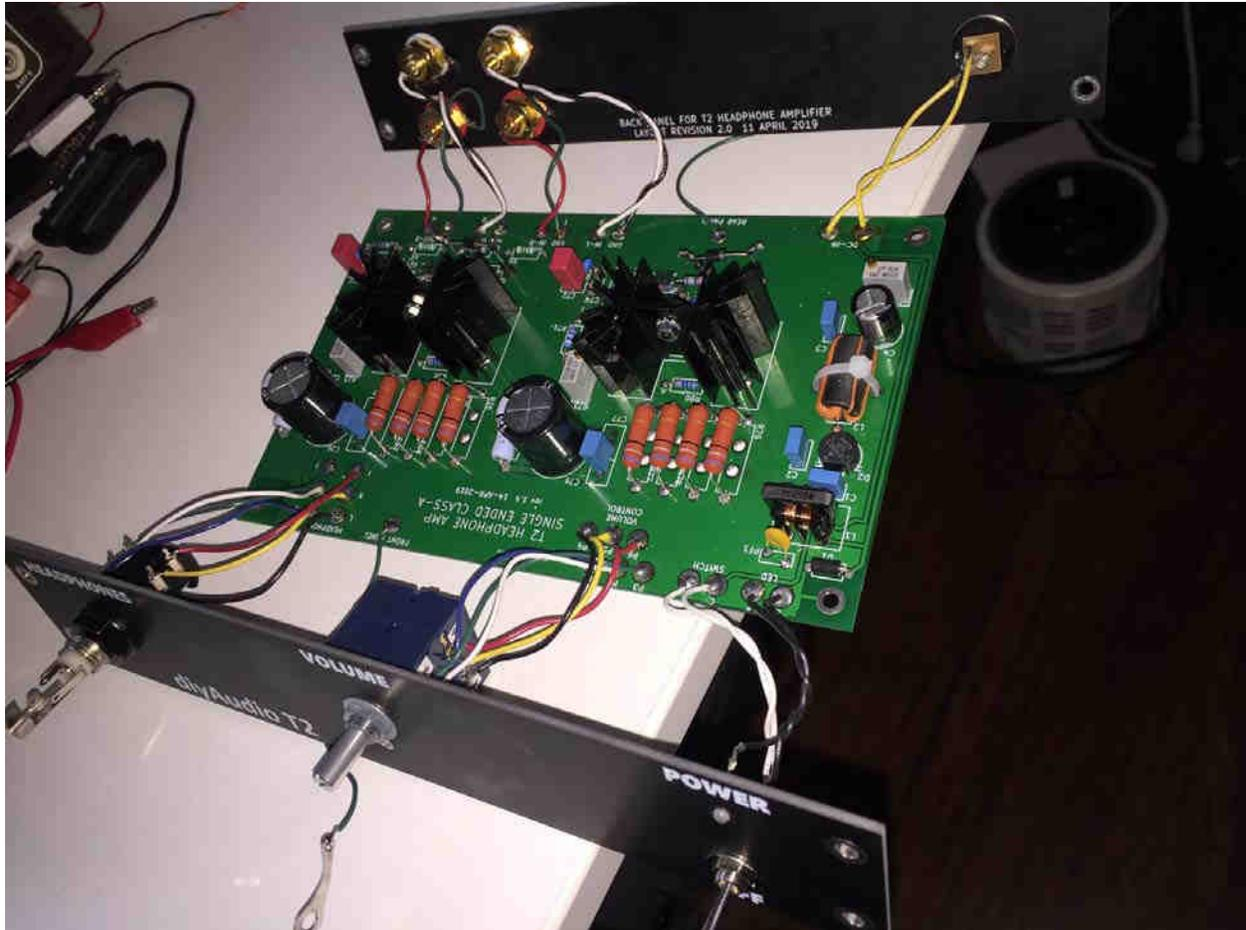
I found it convenient to assemble the PCB, front panel, and back panel completely separate from the chassis. Other builders might prefer another approach.
