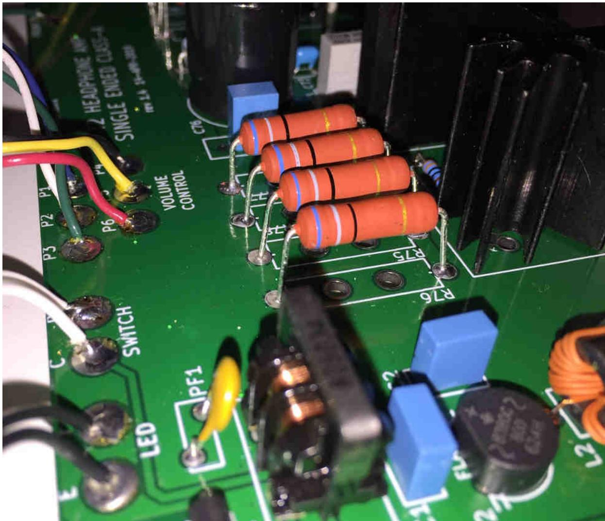
HOWEVER, we need to perform this step early in the build, otherwise it becomes impossible to remove the pencil halves after soldering! You can see that the blue box capacitors and the common mode choke, block the pencils from sliding out. Solution: do the pencil soldering operation before the blocking components are mounted. Like, right after soldering the super low profile resistors and diodes.
