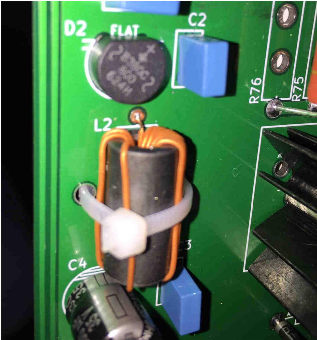
This photo shows the ferrite choke mounted to the PCB. Eleven turns of AWG-28 wire are wrapped around the core. The insulation is stripped from the ends of the terminal wires, and they are soldered to the PCB. Then a zip-tie is threaded through the PCB and pulled snug, to hold the choke securely. The goal is to prevent the mounting wires from having to support the weight of the core, and to make the assembly robust during shipping, rough handling, or vibrations.
