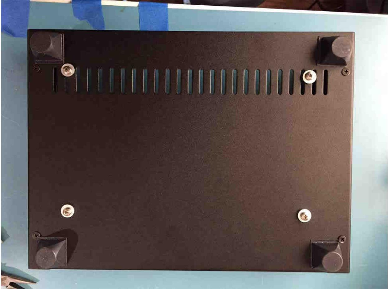
Thus is the outside (exterior) face of the chassis bottom. M3 bolts and shoulder washers are inserted from the outside towards the inside. Tall feet are used to get the T2 chassis far above the tabletop. This improves airflow and reduces the chance of burning or scorching whatever the T2 is sitting upon.
