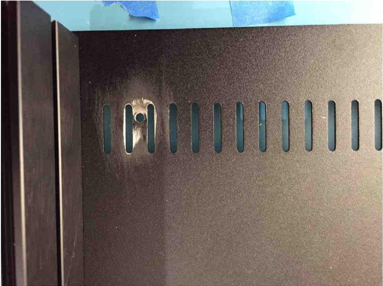
Here's a close-up after drilling and sanding. Do you see that the metal has been deflected (warped) downward? I put a huge stack of newspapers between the metal and the wood when drilling. Big mistake, the newspapers had a lot of "give" but what I wanted was Support. The metal deflected. Oops!
