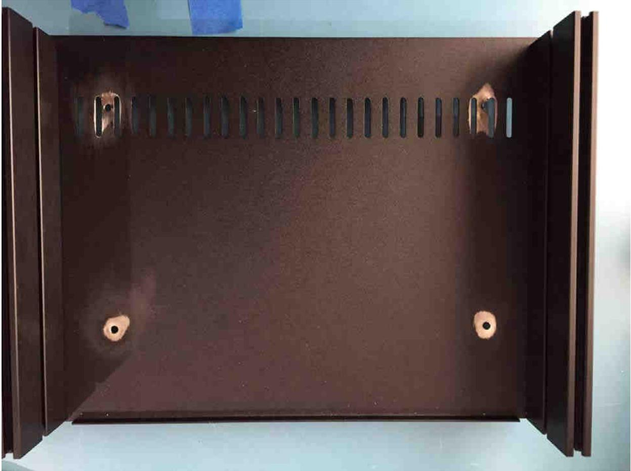
After drilling, use relatively coarse sandpaper to remove the black paint and expose the shiny steel, surrounding the drill holes, on the inside of the chassis. (No need to do it on the outside of the chassis). This exposed metal lets the mounting posts make good electrical contact to the bottom plate, extending the Faraday Cage which surrounds T2 and blocks hum.
