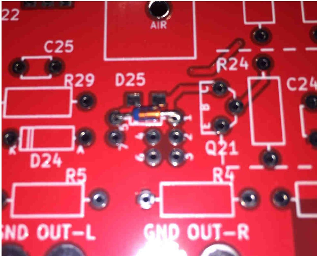
Here is Diode D25 soldered to the PCB. The end with the blue band (the cathode) is soldered in hole#5 and the other end is soldered in hole#1. This photo also makes it abundantly clear that an SMD footprint of the diode (complete with rectangular pads) is present.
