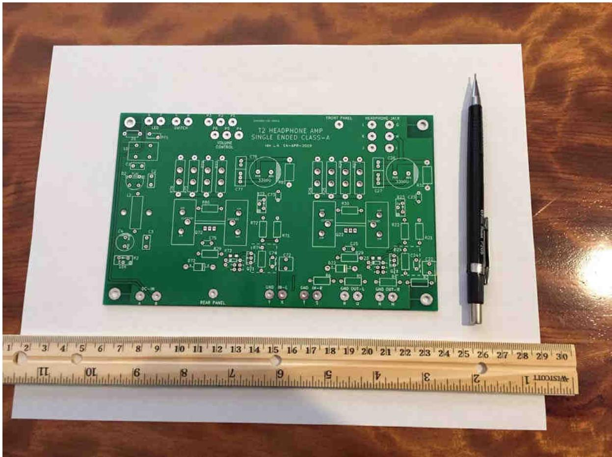
First we'll create a paper template that shows EXACTLY where to center punch the PCB mounting holes on the bottom plate (floor) of the chassis.
