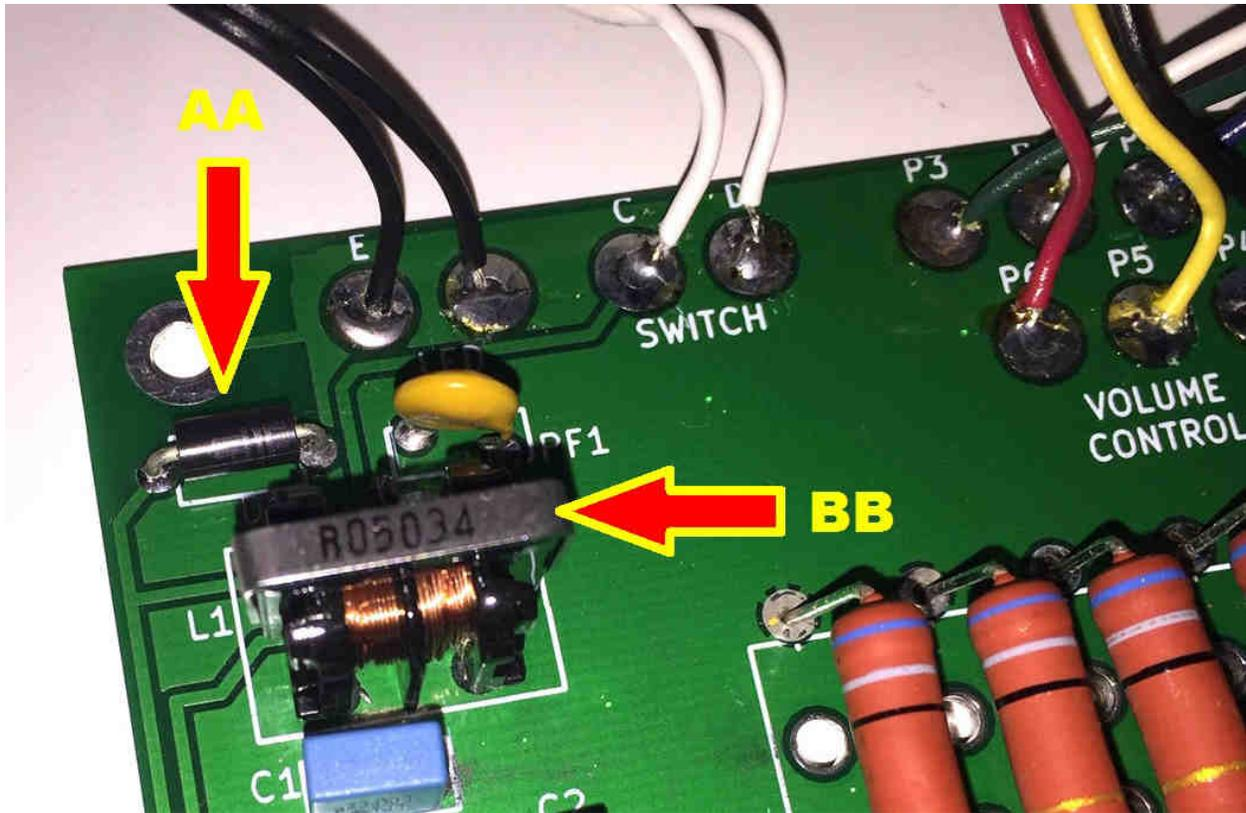
Component D1 is a bidirectional Transient Voltage Suppressor (“TVS”), so it has no white band at one of the package body, designating Cathode. There is no Cathode on a bidirectional TVS. Just like a resistor, you can stuff and solder the part either way; both are equally good. See arrowhead AA in the photo.
