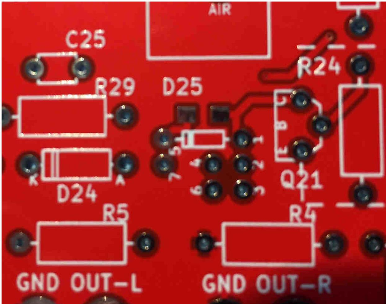
Diodes D25 and D75 have a bit of an unusual “footprint” on the PCB. The plethora of extra pins provides test points (access to interior circuit nodes) and also gives the option to use a surface mount version of the diode, if desired.
