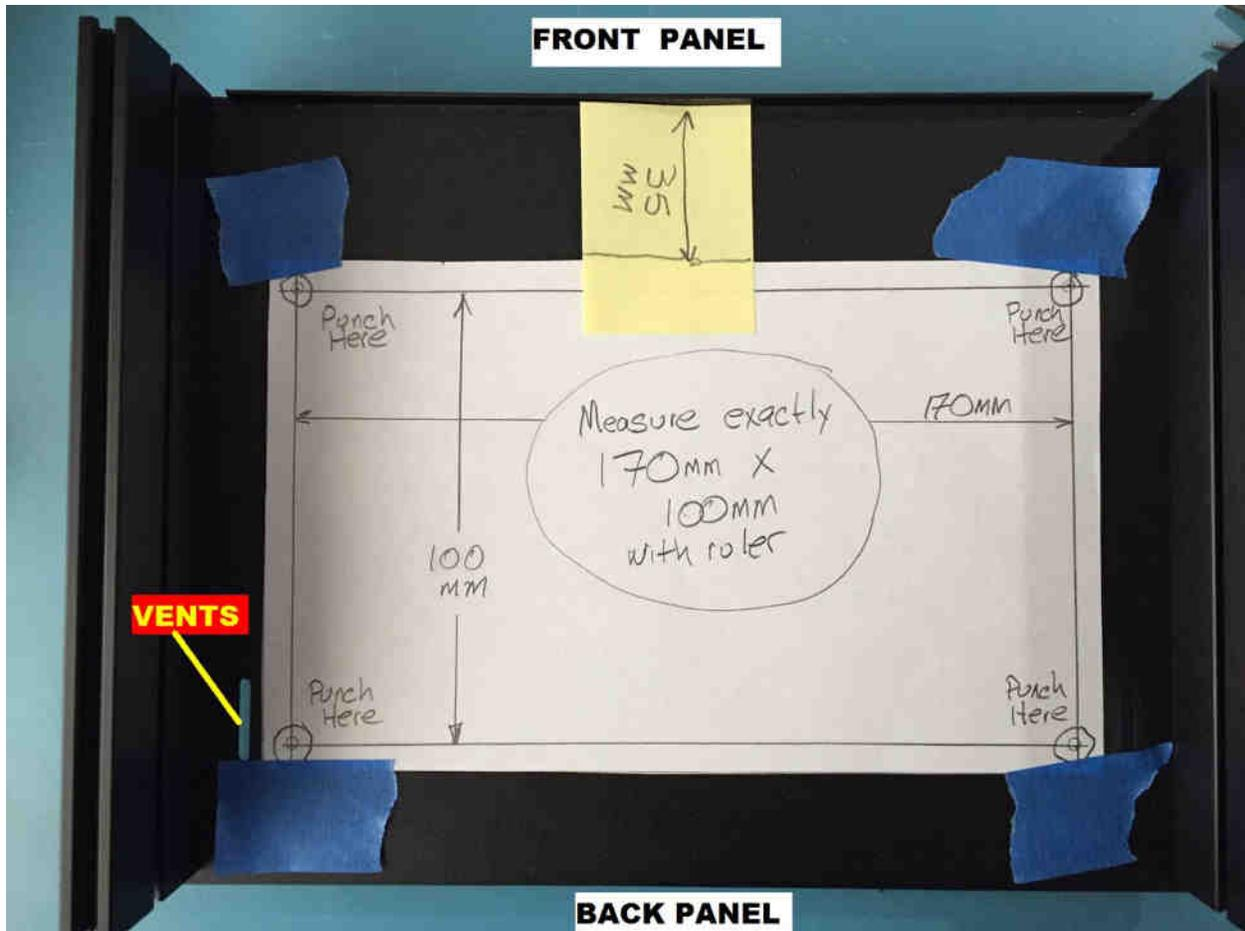
Tape the template to the bottom plate (floor) of the chassis as shown. It should be centered left-to-right, and it should be 35mm from the front panel bent “lip” of the bottom plate.
