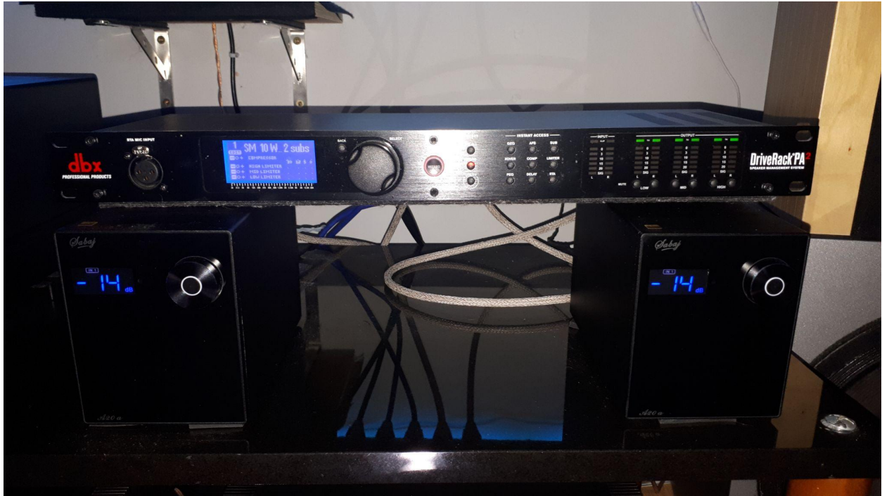
Two Sabaj stereo balanced amps, only using one channel of each amp.
