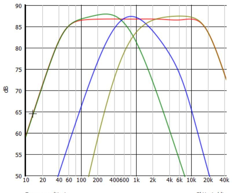
The baffle step  $(0.5+s)/(1+s)$  796Hz for 25cm width has been included.
