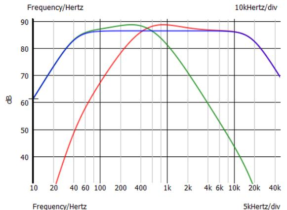
The woofers were limited by the excursion, there is no problem to boost the treble with a bigger amp, but the tweeter would not allow the boost because of thermal limit.
