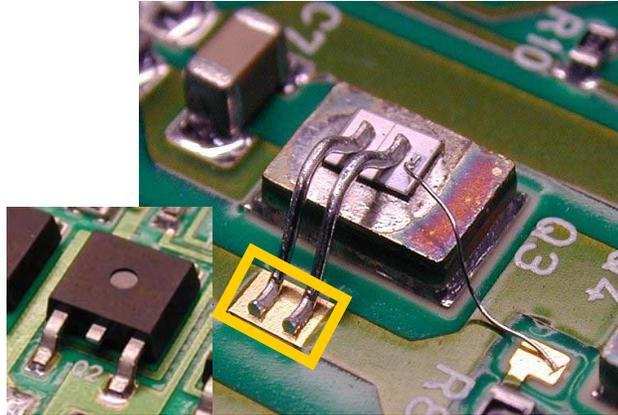
*Conventional transistors are packaged in plastic with prefabricated leads (left). To achieve the shortest possible signal path, Sony uses bare MOS FETs and employs molecular bonding to connect each lead to the circuit board. The bare transistors and their connections are then encapsulated for protection.*
