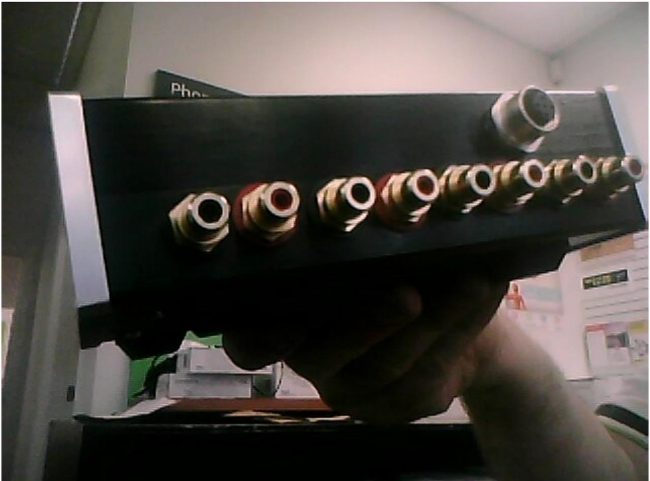
The rear panel carries from the far Right referring to the above image RCA sockets for Outputs Left and Right , followed by Input 1, left and right, followed by Input 2 and to the far left Input 3, ( Input 3 being selected when the front panel knob is furthest to the right of its travel )
