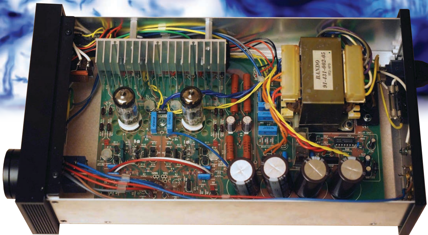
Photo 1: The modified Stax SRM-T1 has increased drive capability and sound quality.
