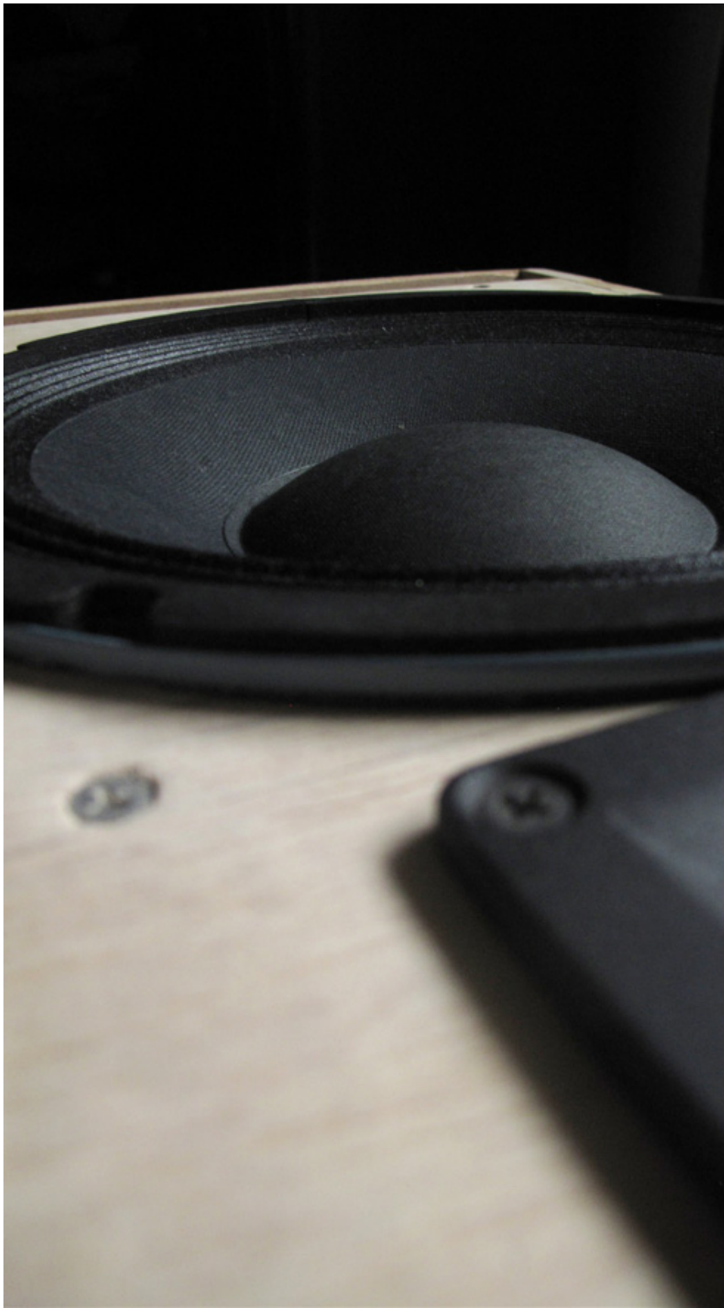
A 10” mid woofer produced for the pro audio market matched to a Compression driver. The aim of this design is to produce a full range speaker that has a clear dynamic sound. In many respects this project is a work in progress.
