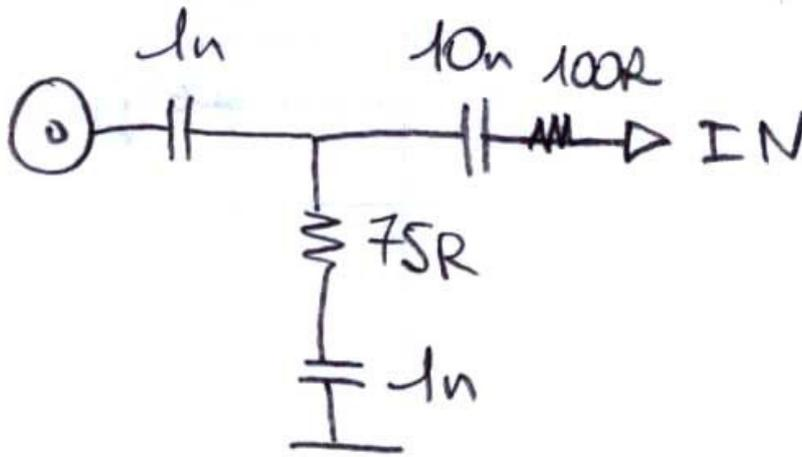
The  $1nF$  cap is in series with the cap inside the transmitter, since it is smaller, it dominates it. The termination network ( $75R+1n$ ) forms a divider. This is a bit like a 10x scope probe.
