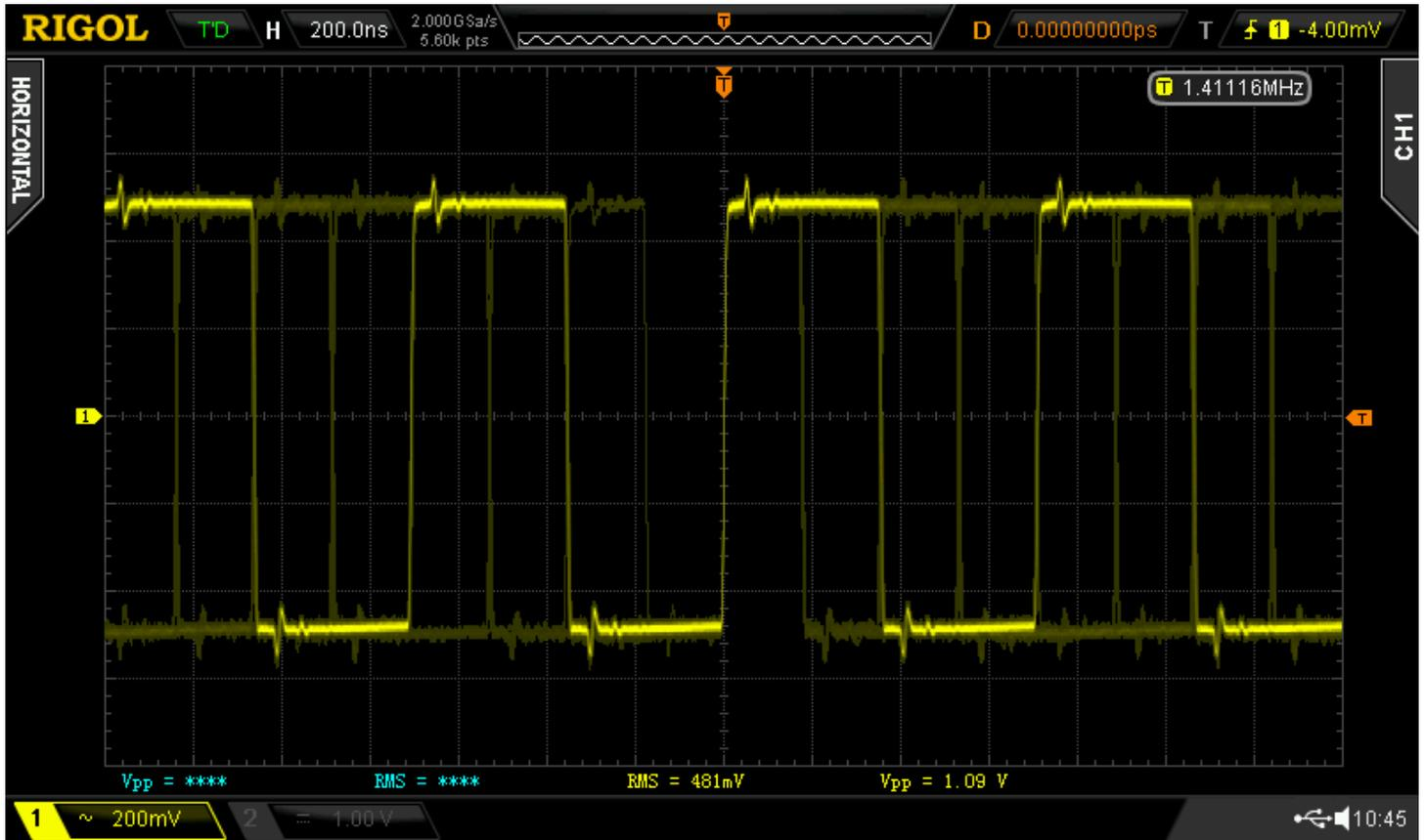
CT=Short : transmitter AC-coupling cap distorts waveform.
