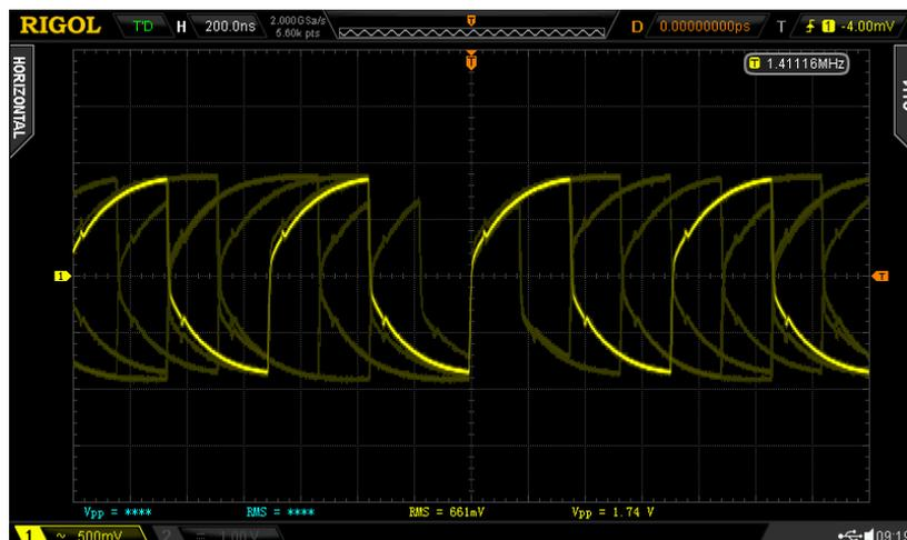
So, AC-coupling the termination resistor seems to have useful effect, but there is a gotcha, the AC coupling cap should be about the same value as the coupling cap in the transmitter ...
