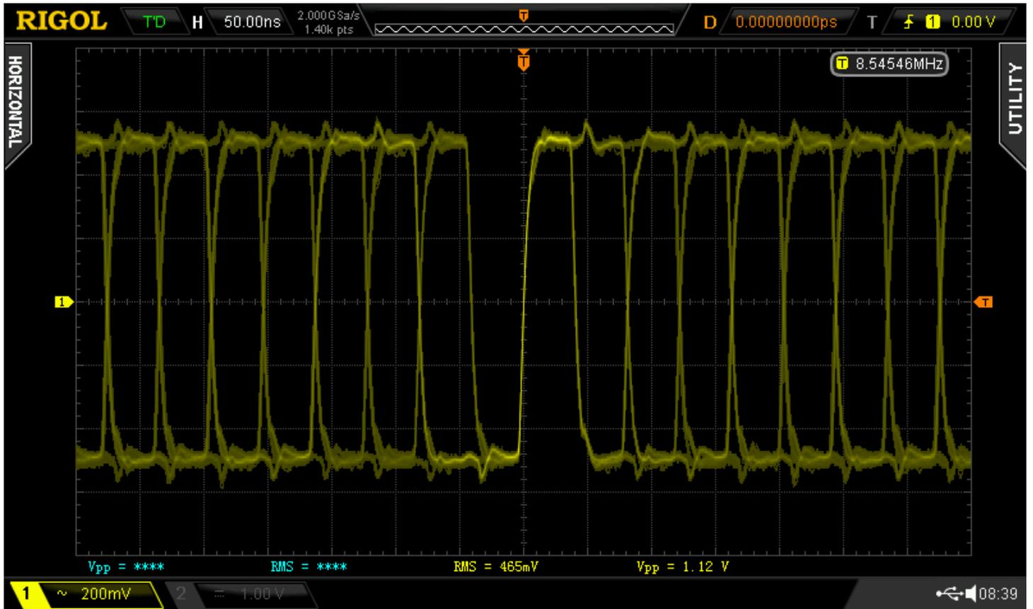
At 44k, it is visible that the coupling capacitor in the SPDIF transmitter creates a highpass with termination resistor on my end of the cable, which adds data-dependent jitter :
