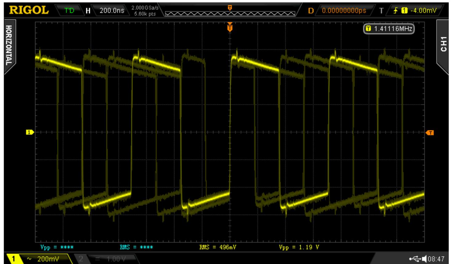
A bit of calculation : the slope looks like the transmitter has a 22nF cap in series.
