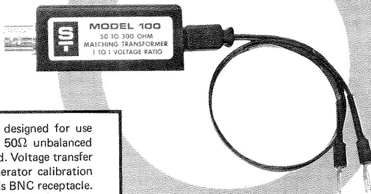
The Model 100 Matching Transformer, designed for use from 54 MHz to 216 MHz, converts a 50Ω unbalanced signal generator output to 300Ω balanced. Voltage transfer ratio is 1:1 ± 10%, retaining signal generator calibration into a 300Ω load. 50Ω input connector is BNC receptacle. Detachable 300Ω output plug is wired with 12" of twin lead terminated in spade lugs.
