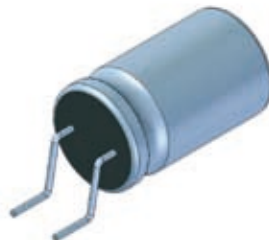
Oberflächenmontage leads prepared for surface-mount
