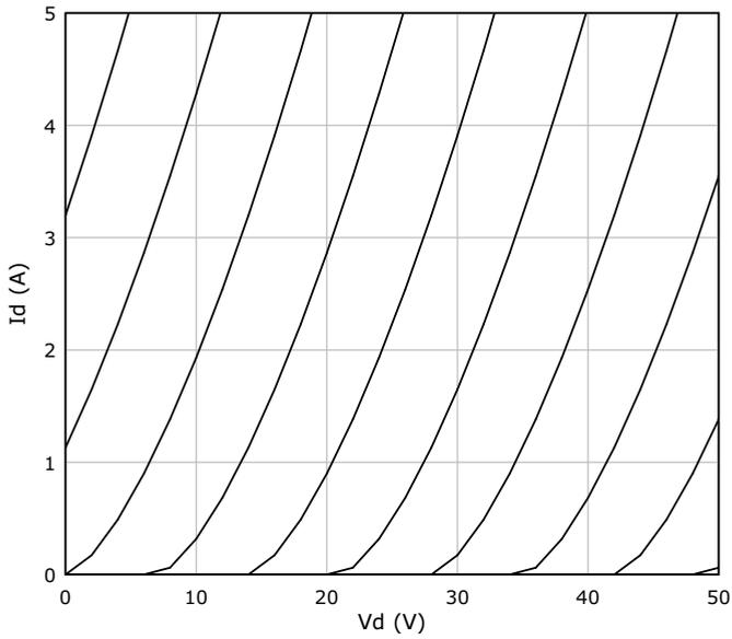
Figure 2 Power SIT curves based on equation (2)
