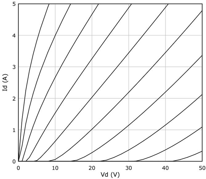
*Figure 5 2SK82 curves based on eq. (5).*
