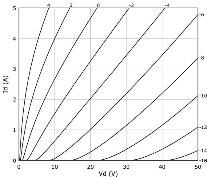
Figure 7 2SK82 curves from SPICE based on eq. 5.
