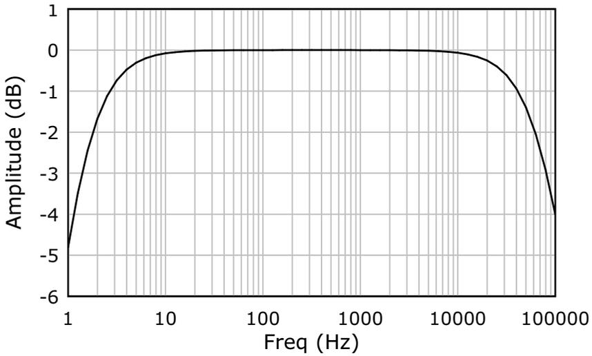
Figure 9 Frequency response of figure 8 test circuit.
