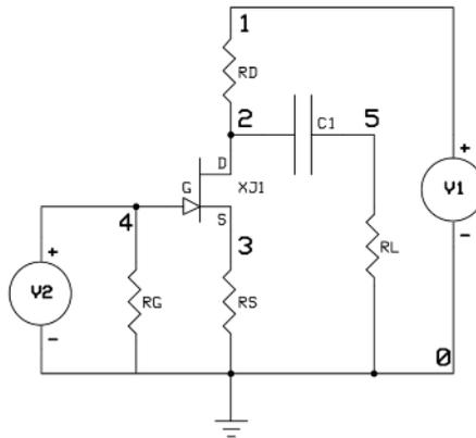
Figure 8 2SK82 SPICE common source test jig.
