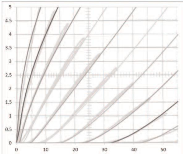
*Figure 6 2SK82 curves based on eq. (5) overlaid on curve tracer output.*
